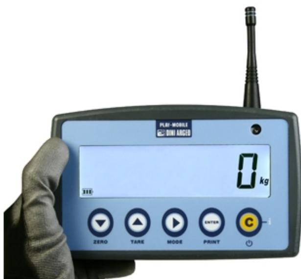
Radio frequency weight repeater for DFW indicators and MCW crane scales, easy to transport and view thanks to its small size and to the backlit large digit display. It allows to repeat the main scale functions from a distance, thanks to the integrated keypad, and to memorise the weighs for the following processings by PC through the serial commands or the "Weigh Console" software
