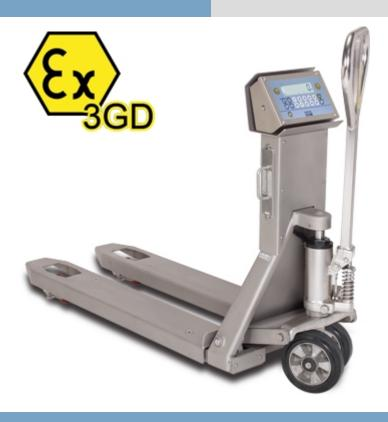
Pallet truck scales, with built-in electronic weighing, suitable for harsh working conditions and dangerous areas classified as hazardous (ZONE 2, 22) in accordance with Ex II 3GD IIC T6 T130°C X protection. The weight detection made with four Atex certified IP68 stainless steel load cells guarantees the precision in all work conditions. Structure entirely in stainless steel. Available also CE-M APPROVED.
